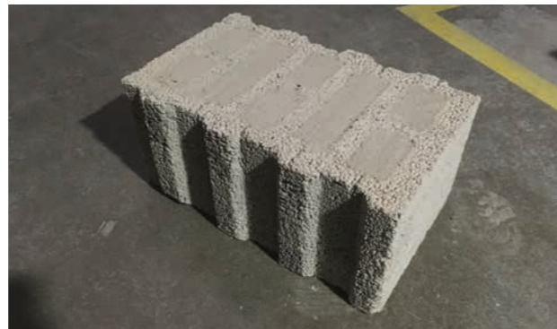
Example of a filled concrete block with insulating foam 33 mW / m*K
