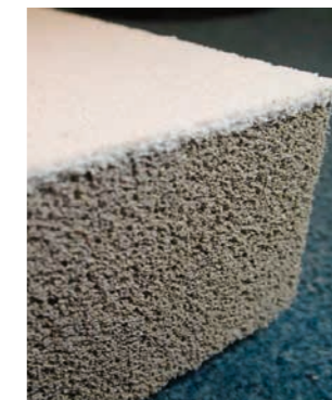
The pores in the microstructure offer excellent sound-proofing and heat retention properties.
