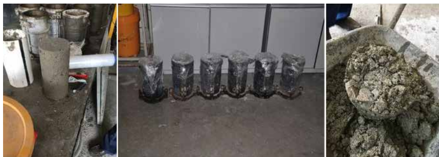
Figure 3.3.1.1: Laboratory trial cylinders of RCC
