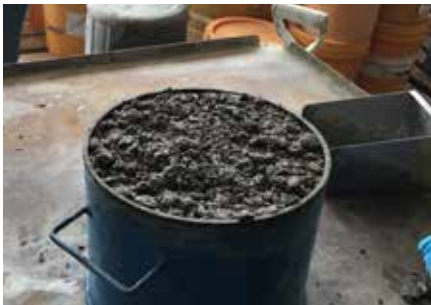
Figure 4.2.1.1: A sample of RCC (“concrete approach”) before Vebe testing
