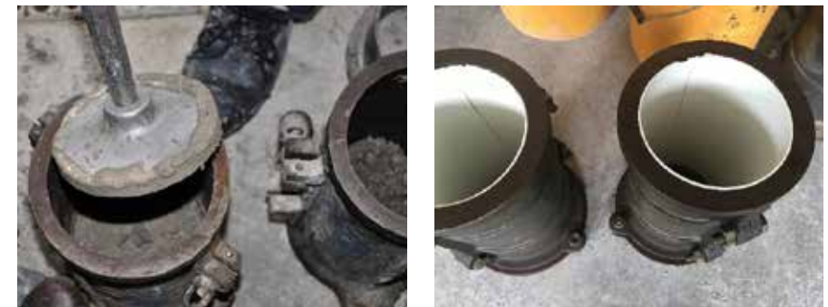
Figure 4.3.1.1: Steel moulds (on the left) and single-use plastic moulds with steel sleeves (on the right)
