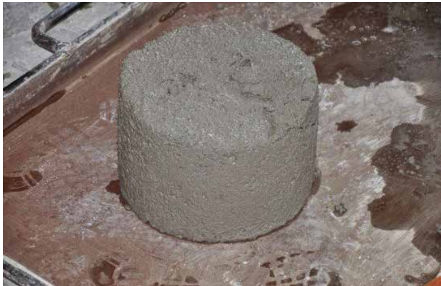
Figure 4.2.1.4: RCC sample after consolidation with Vebe apparatus
