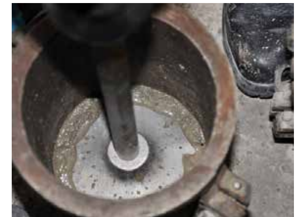
Figure 4.3.1.3: An example of vibrating compaction hammer (on the left) and of the moment when mortar paste came up around the total perimeter of the circular steel plate (on the right)
