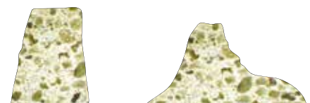
Figure 1.1.3: Forms of slump
