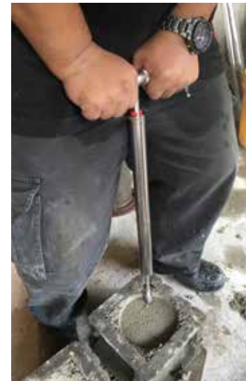
Figure 4.2.5.1: Reading of a penetration test on a RCC specimen
