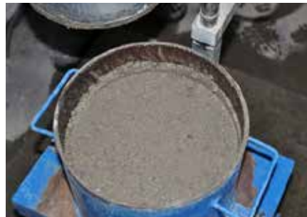
Figure 4.2.1.2: A sample of RCC (“concrete approach”) after Vebe testing
