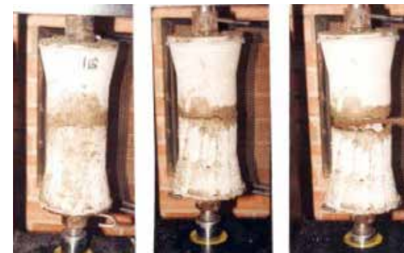
Figure 4.3.3.1: Specimens to measure the direct tensile strength of horizontal joints from an RCC with low-cementitious material
