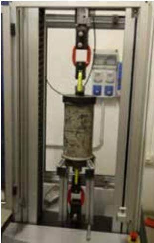
Figure 4.3.2.1: Tensile strength test on a cylindrical specimen of RCC
