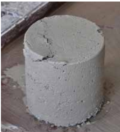
Figure 4.3.1.2: RCC sample after consolidation with Vebe apparatus
