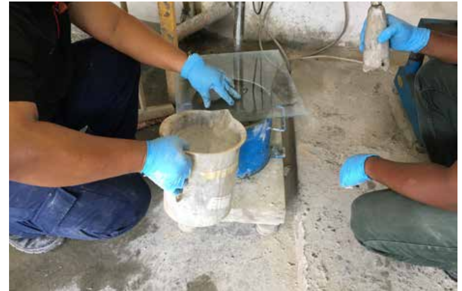
Figure 4.2.2.1: The determination of the total mass of the cylindrical mould, consolidated specimen, water and flat plate
