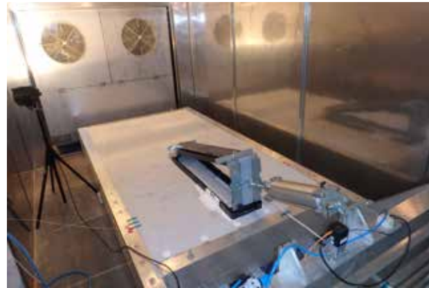
Horizontal load testing of an SSM1 mount in a climate chamber
