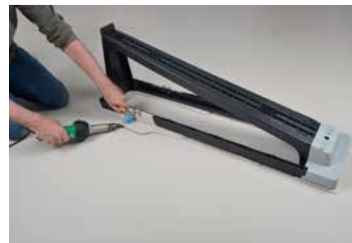
Hot-air welding of a Sika® SolarClick flange
