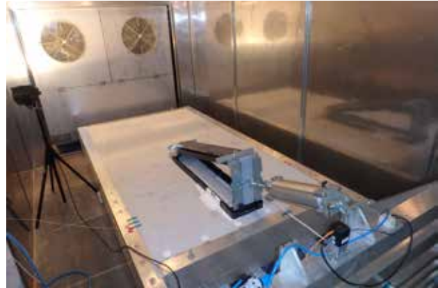
Horizontal load testing of an SSM1 frame in a climate chamber
