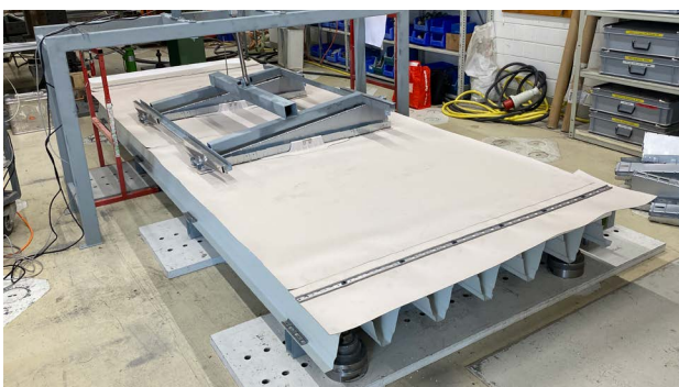
Mechanically applied uplift loads to a PV module on two SSM2 mounts
