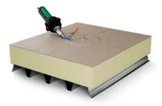
Hot-air weld the SikaRoof® Anchor 250 CR onto the roofing membrane according to the Sika Roof Application Manual.
