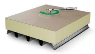
Screw-on the SikaRoof® Anchor 250 CR on the SikaRoof® Anchor Washer 140 and tighten with a spanner no. 19.
