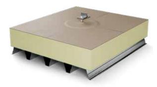
Install the Alu-Adapter plate, the Climber 36/50 with a M12 x 25 stainless steel fastener including washer.
