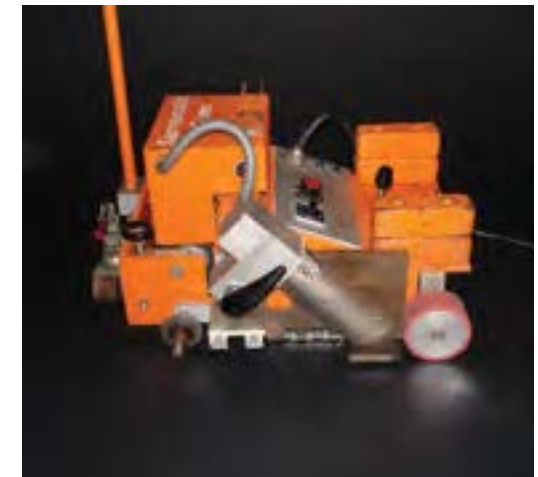
1966, Invention of Sarnamatic® Seam Welder: Sarnafil® was the first membrane manufacturer to design and produce an automatic seam welder, recognising early on that seam integrity was critical to the long-term performance of thermoplastic roofs.
