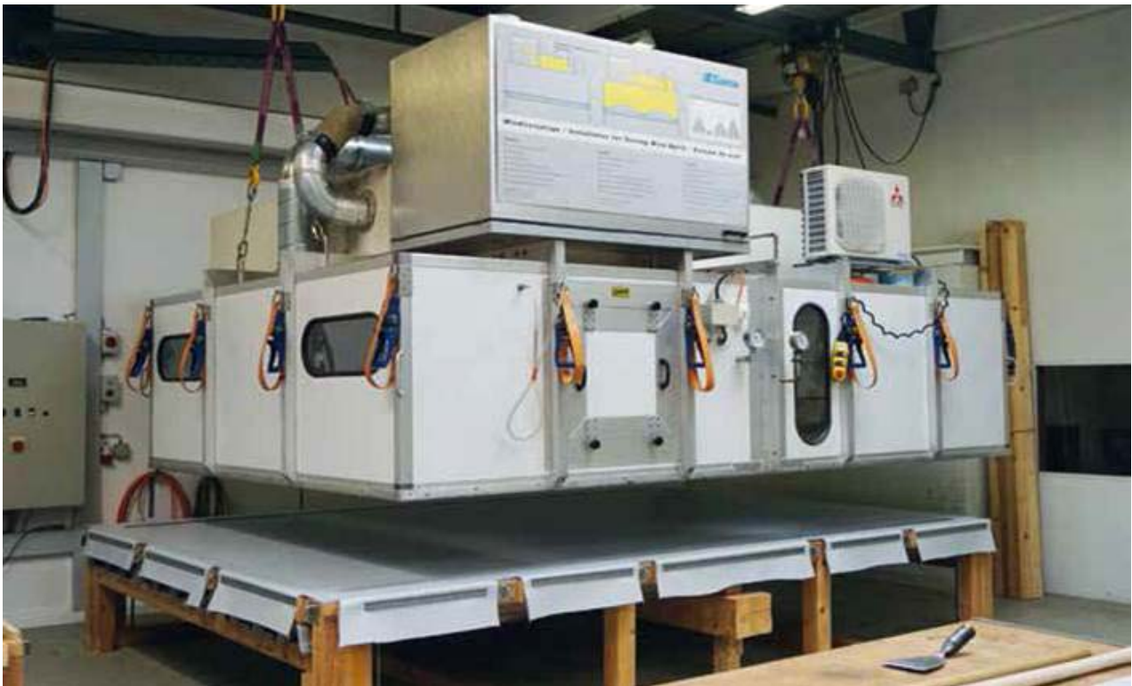
Wind-uplift test facility
