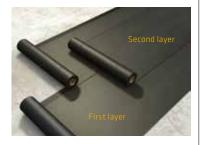
If the layers do not adhere well to each other, the water can pass through the innumerable "channels" existing. The security of a multi-layered membrane is ensured exclusively by the complete adhesion between the layers, which make it up.
